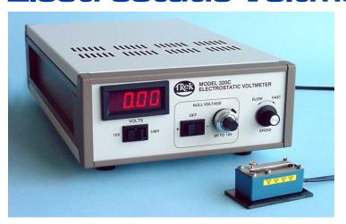
The Trek Model 320C Electrostatic Voltmeter is a versatile instrument which is used for a variety of electrostatic applications including contact potential measurements, materials evaluation, and electret studies. The Model 320C makes highly accurate, noncontacting measurement of electrostatic potentials of 1 mV to 100 V over a wide range of probe-to-surface distances. The Model 320C is specifically designed for high sensitivity applications.
