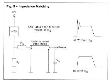
strength of standard coaxial cable is usually specified for high frequency. Here the DC-voltage strength which is of more interest lies generally about Factor 4-8 higher. If there is any doubt, the cable should be tested for its voltage before being used or else the cable manufacturer should be consulted.
