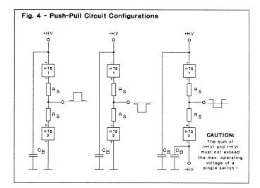
Since HTS transistor switches are fitted with protection circuits which work independently, parallel or series operation should be done only in exceptional cases and then only with the greatest care.
