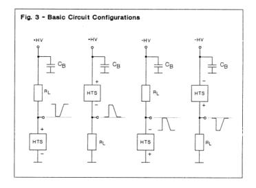
Figs. 1 to 4. The line paths should always be kept as short as possible and the high-voltage supply should be buffered as near to the switch as possible by means of a sufficiently large capacitor  $C_B$ . Otherwise dangerous flyback voltages might be induced on unbuffered lines (cf. 7.3) or load capacitances might not be charged or discharged fast enough. In the case of push-pull circuits it is vital that series-protection resistors are used, which limit the load
